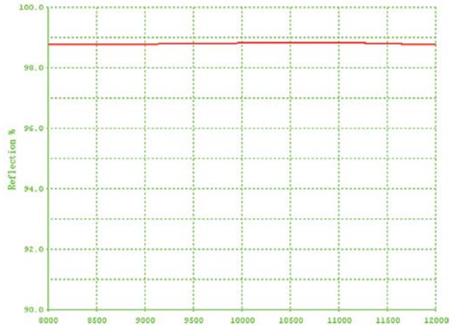
Au Reflecting Metal Coating 8 μ m--12 μ m
