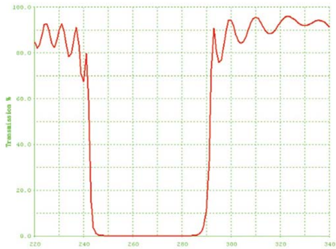
Single Wavelength Dielectric High-reflecting Coating 266nm
