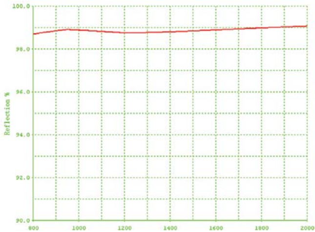
Ag Reflecting Metal Coating 800nm--2000nm
