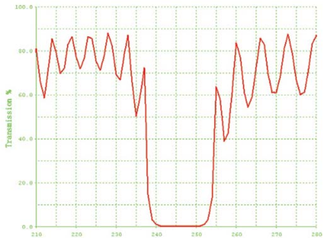
Single Wavelength Dielectric High-reflecting Coating 248nm
